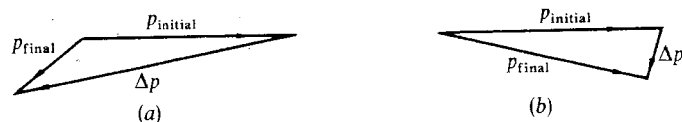
Fig. 2.19. Change in linear momentum of bombarding electron (a) Small impact parameter (b) Large impact parameter.
