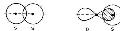
Fig. 6.6. Overlap between two s orbitals, and one p and one s orbital
